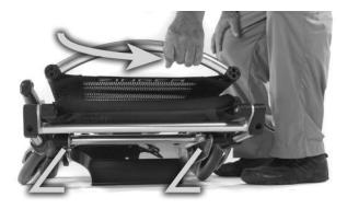
There are many occasions in which you will need to lay the Zinger on the floor. First fold the Zinger as described on the previous page. Next lower the Seat Back Bar until the Front Caster Wheels begin to contact the ground. At this point apply a rotational motion (top arrow) as you lower it further, so that the Front Caster Wheels both lie down together in the same direction. If you do not use this rotational motion the caster wheels may stand up thus preventing the Zinger from lying flat.
