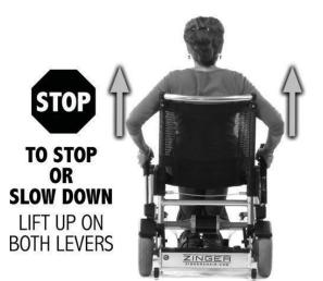
**NOTE:** Remember that the brakes will always apply when both levers are pulled back. If you have any confusion, just pull up on BOTH levers to brake!
