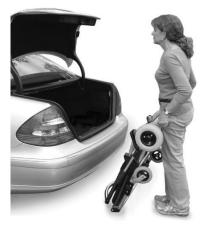
Grab the Anti-Tip Wheels and lift the rear of the Zinger so that it leans against your upper thighs as shown.
