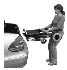
Next, grab the Cross Tube to lift the Zinger off the ground with the Battery cradle pressed against your thighs.
