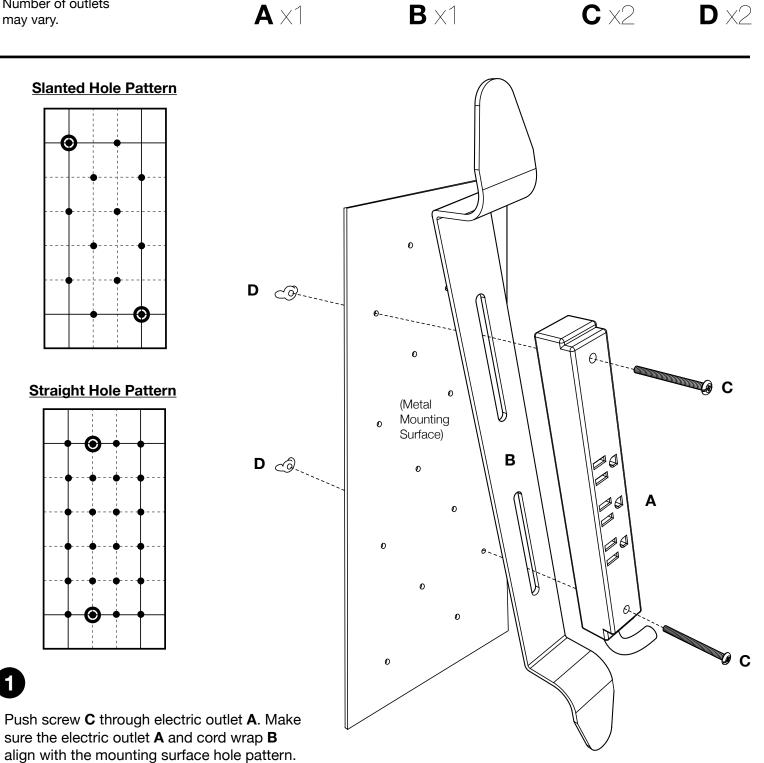
Push screw **C** through cord wrap **B** and the mounting surface screw holes. Use wing nut
