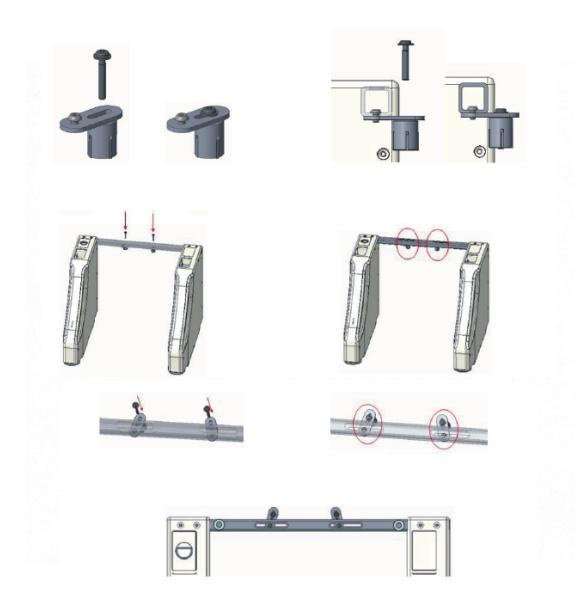
Shown above, clockwise from top-left: The toilet brackets and expansion bolts. A cut-away of the rear support with the bracket bolt installed. The location for the brackets on the rear cross member An example of how the brackets install. Another view showing that the bracket bolts go into the slot. An illustration of the expansion bolts and how they go through the bracket. Arrows showing the installation of the expansion bolts from above. (this is done when you install the lift on the toilet).
