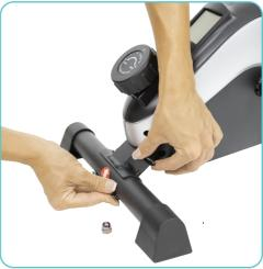
2. Attach the Rear support Pipe to the Main Frame by aligning the screw holes on both parts and inserting two Carriage Screws into the holes with an Arc Washer and Cap Nut on the side nearest the Main Frame. Tighten the nuts securely with the included wrench.
