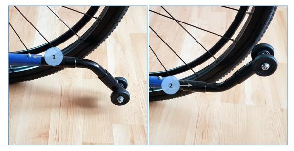
If the wheelchair is to go up or down a high step (e.g. a curb), the anti-tip wheels must be swivelled upwards to avoid them catching on the ground. Pull on them to unlock (2) and swivel up/down so it looks like picture 2 above.
