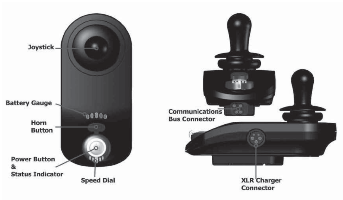
Figure 36: The Remote REM050: user interface and connectors
