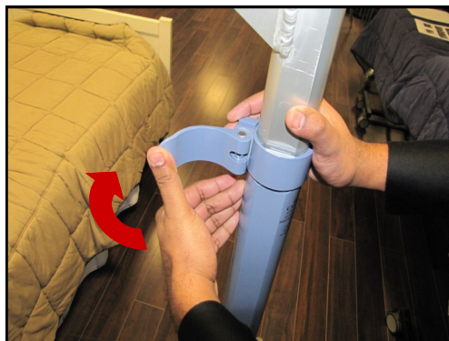
Step 2 - Fully open the clamp.
