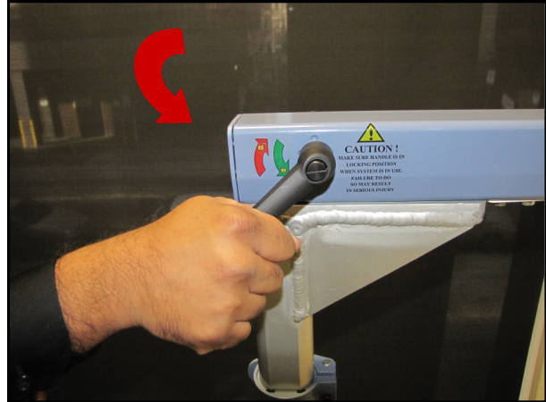
Step 13- Twist the handle downwards in the lock direction.
