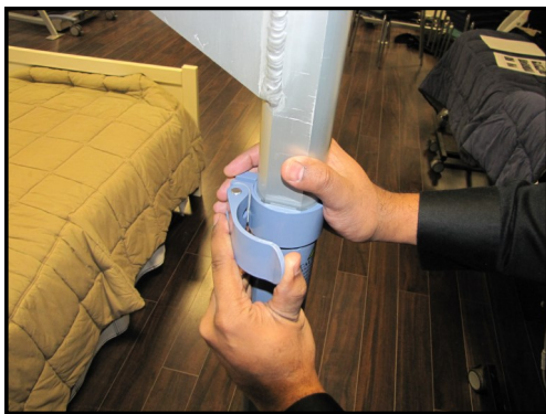
Step 1 - Grab the post center to open the post clamp.
