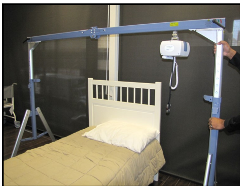
Step 5 - Repeating steps 1-5, raise the opposite post.
