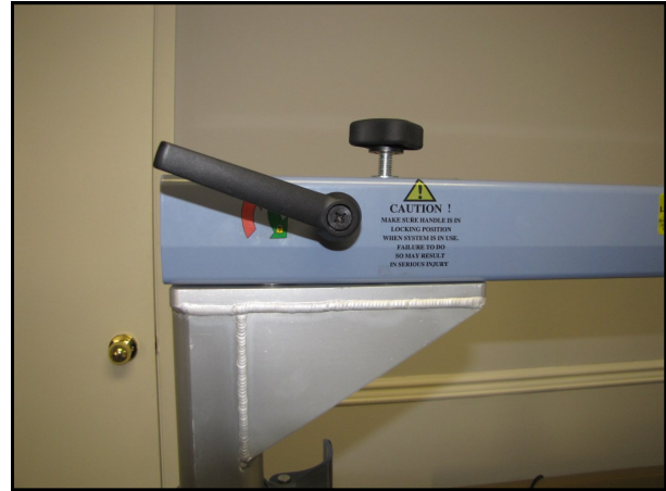
Step 9 - Hold plastic knob up and place track on post.
