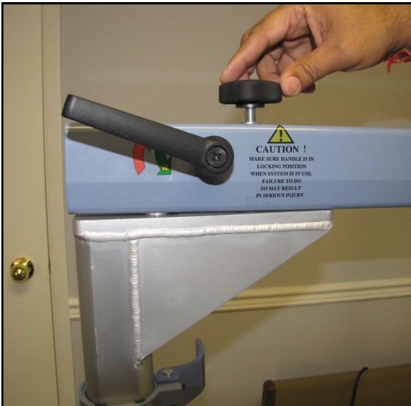
Step 10 - Turn the plastic knob clockwise so that the track locks with top post.
