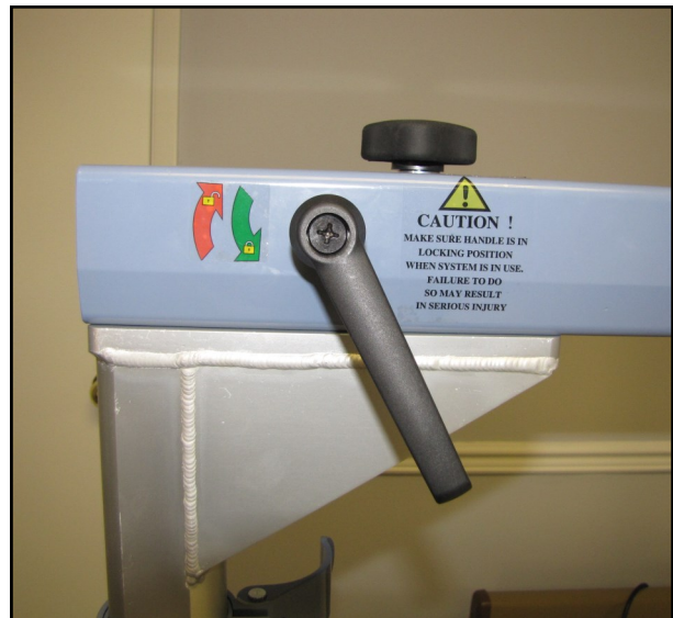
Note: Above picture shows that the plastic knob is flush with track, and track locked with top post.
