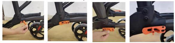
4. Press down from both sides of the seat to open the frame. A click will be heard once it is locked. ALWAYS ensure the seat is locked before sitting on it.
