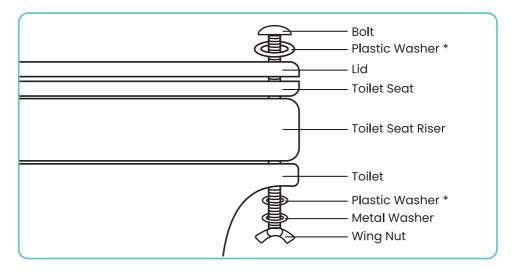
**Note:** Plastic Washer placement may vary. Place the plastic washer above the lid if needed to secure the head of the bolt. Otherwise, place plastic washer between toilet and metal washer.
