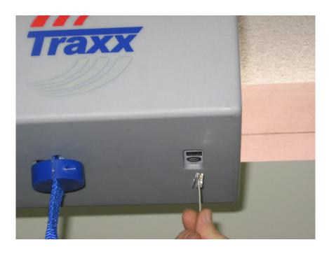
Connect Remote Control by plugging into control panel. Next, place Lift Bar on bed and lower Lift Belt to connect them together.
