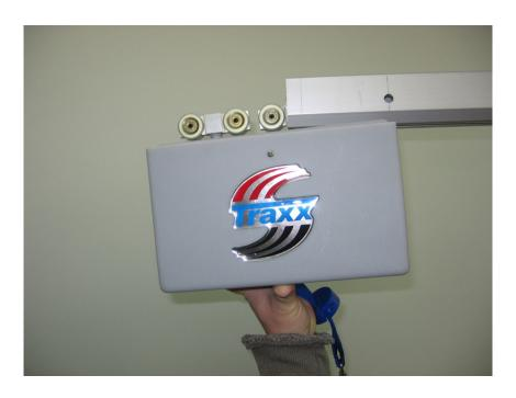
Carefully install Lift Motor by sliding trolley wheels into bottom channel of open end of Transverse Beam. Roll Lift Motor to other end of frame. Be careful not to let Lift Motor roll out open end and fall.
