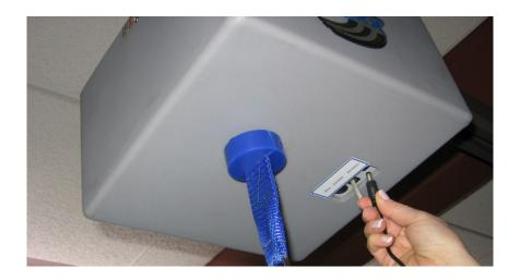
Plug Battery Charger in Lift Motor and outlet and charge battery overnight prior to first use. Always unplug the charger before using the motor.
