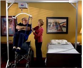
Lift patient with Remote Control above wheelchair or other device. Adjust Sling if necessary. Slide patient in Sling over center of bed and lower with Remote Control until sitting or lying comfortably and safely on the bed. Maintain control of Lift Bar until safely up and away from the patient's head and face. Remove Sling carefully from under patient by gently rolling them from one side to the other. Use bed rails if available.
