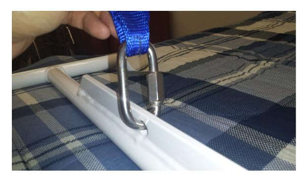
Hand tighten Link to close completely. Raise Lift Belt and Lift Bar to Motor Housing.
