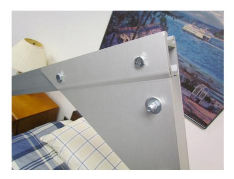
Install two 3/8" x 3 1/2" bolts with nuts. Do not tighten nuts completely at this time.
