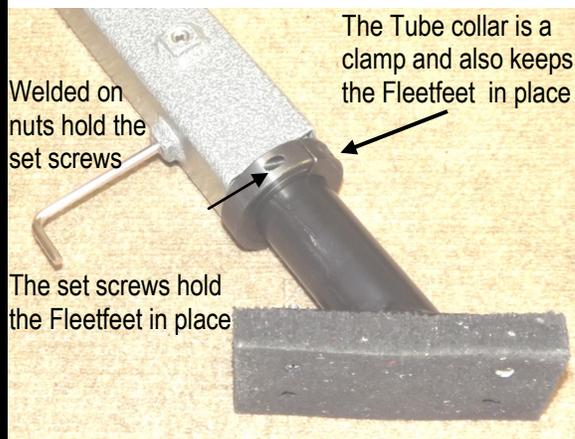
You can remove the 4 bolts and use the holes in the plate and rubber mat to fasten firmly to almost any floor
