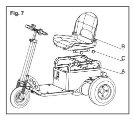
**4.8 Assemble Tool Box (See Fig. 8)** Assemble the Tool Bag (B) to the rear of the Frame (A).
