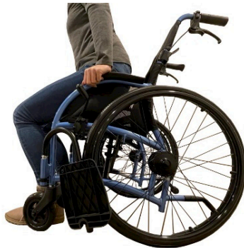
Figure 6 Correct posture – centre of gravity in the centre and front wheels facing forward.
