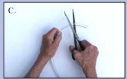
A common household scissors (photo "C" above) is all that's needed for the installation – to cut the transparent  $O_2$  piping to the desired lengths for your individual home layout.
