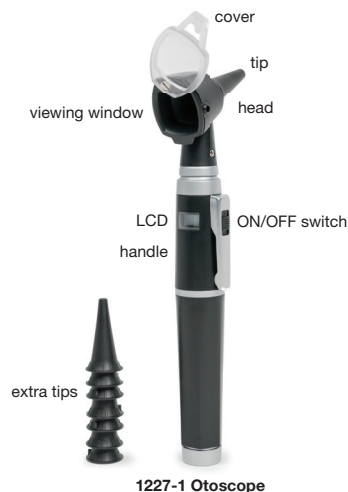
The Graham-Field 1227-1 Otoscope is shown above with features labeled.
