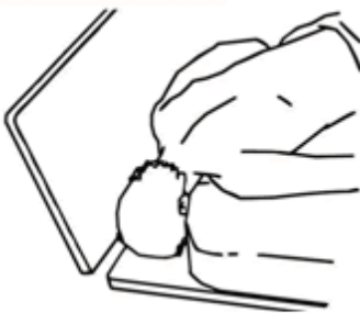
Zone 7 - Entrapment between head or foot board and the mattress end
