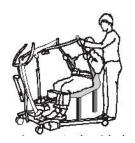
5. Attach appropriate length back straps to the carry bar/yolk. It is very import-ant that the chosen length strap does not disrupt the client from a comfort-able sitting position. (Shoulders should remain in line or slightly behind the hip, straps that are too short will cause the client to lean, inappropriately forward).
