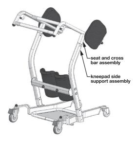
6. Insert the seat and cross bar assembly into the tubes at the top of the kneepad side support assembly as shown above.
