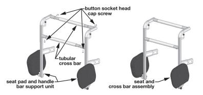
4. Insert the two tubular cross bars into the holes on the seat pad and handle bar support units as shown above. Align the small holes on the cross bar undersides with the holes in the support units. Install the four button socket head cap screws through the support units into the cross bars. Use the hex key to tighten. The finished assembly is shown at right above.
