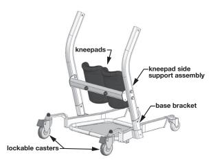
5. Insert the kneepad side support assembly into the base brackets as shown above. The kneepads and arm curvature should be facing away from the lockable casters.
