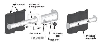
2. Insert the kneepads into the kneepad support unit. Install the two hex bolts through lock washers, flat washers, and kneepad support unit into nuts as shown above. Tighten securely with the provided wrench. Install the two plastic caps on the hex bolts. The finished assembly is shown at right above.
