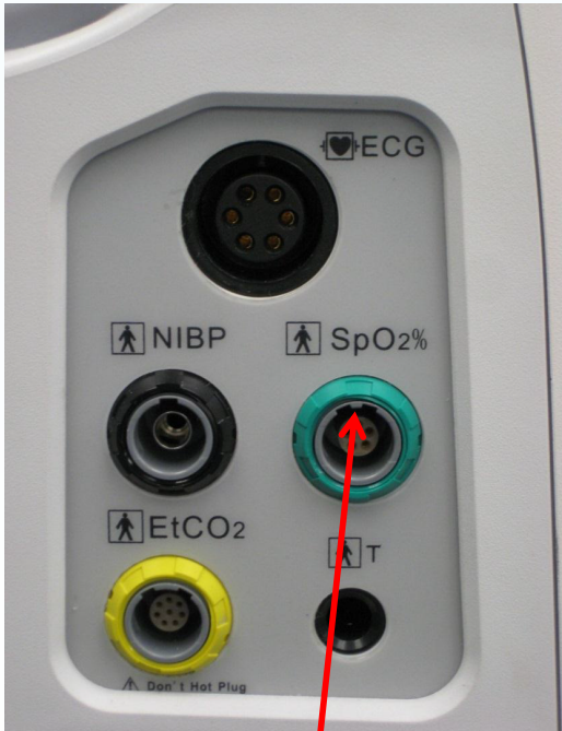
Digital SpO2 Monitors - 2 Keyway Guides; 5 pin connector
