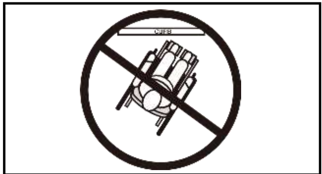
Figure 3. Incorrect Curb Approach
