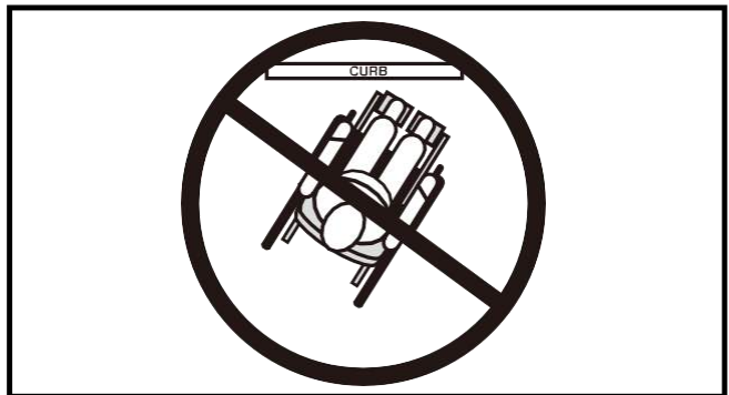
Figure 3. Incorrect Curb Approach
