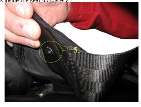
6. Install the screw back into the cross brace and tighten.
