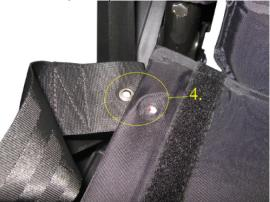
5. Insert the seat screw through the seat upholstery then the seatbelt. It is important to make sure the screw goes through the seat stay that is inside the seat upholstery.
