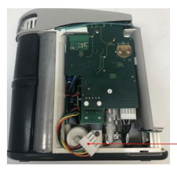
**Compressor Assembly Wires**
