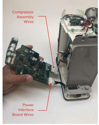
9. PC board (508552) should be able to be removed from unit.
