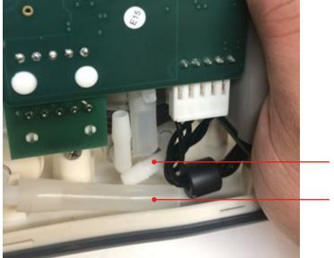
Compressor Pressure Inlet Elbow
