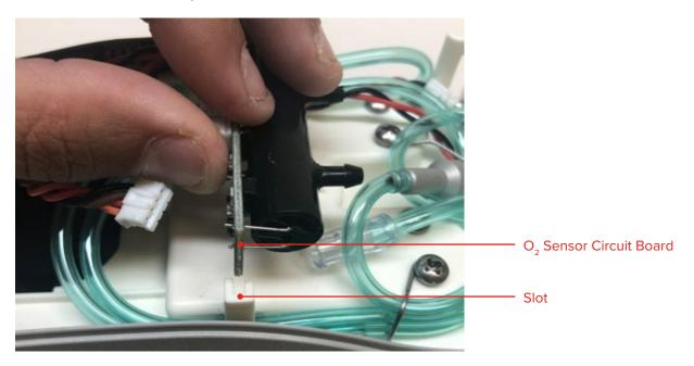
2. Slide the O2 sensor into the slots and press until the O2 sensor locks into place with the locking tab.
