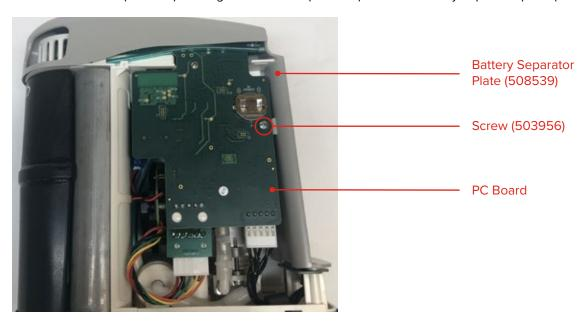
3. On the bottom of the PC board, disconnect the wires from the compressor assembly (508525).
