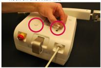
4. Untighten the two screws with a torx screwdriver (TX10) holding the covers together (about 6-7 laps or until it's loosened). The screws are located at the bottom of the holes for the rubber feet/plastic.
