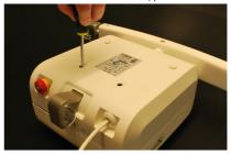
5. Turn the lift around and remove the cover by angle it a bit towards the hanger bar until you hear a "click".
