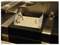
3. Unscrew the two metal brackets from the chassis by using a 2,5 mm Allen key.
