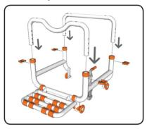
Insert both height adjustment tubes into the base legs. The height adjustment tube with the 'U' bend should be inserted into the front.
