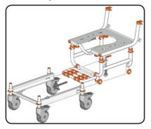
With the wheeled base track assembled on a flat surface apply the brakes on the 4 castor wheels.
