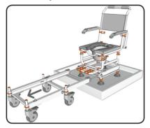
With your Showerbuddy secured in position on the shower base remove the bridge and wheeled base.
