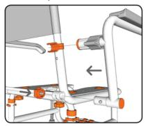
Insert the arm rests into the sockets on the seat base until the clip pin clicks and locates the arm rests in position.
