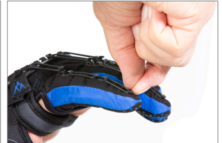
Fig. 32 Reattach DIP Tensioner for all fingers
