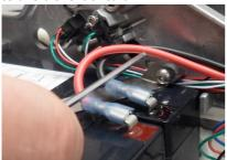
3. Now - disconnect the battery cables located on the battery.
