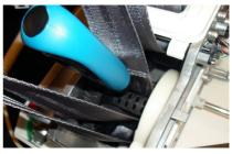
7. Return the belt roll with help of the Roomer S switch or the hand control. Grab the belt.
