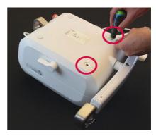
5. Turn the lift around and remove the cover by angle it a bit towards the opposite side of the control panel until you hear a "click".
