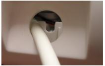
Pull the cable and the connector out through the hole. If the hand control is damaged, you can cut the cable and it will be easier to pull out.
