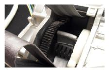
Note! Do not turn the Roomer Switch without holding the belt roll since the spring will unwind. If you drop the belt roll, rewind the belt roll 9,5 turns from the belt roll slot with a metal pin.
