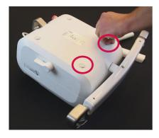
4. Untighten the two screws (TX10) holding the covers together. The screws are located at the bottom of the holes for the rubber feet.
