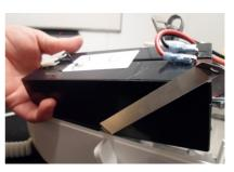
5. When the batteries is removed from the lift, disconnect all four cables.
