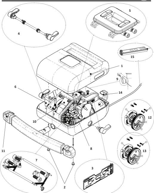
All spare parts for the overhead lifts are sold as a kits. circled and pointed parts shows the kits that are available. Detailed list with included parts is shown at the next page.
