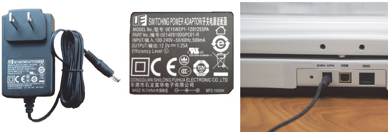
Figure 3-4. Outlet and AC Power Connection Site on Back of Scale
