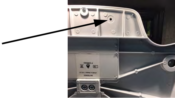
Figure 4-1. Setup Switch Location
