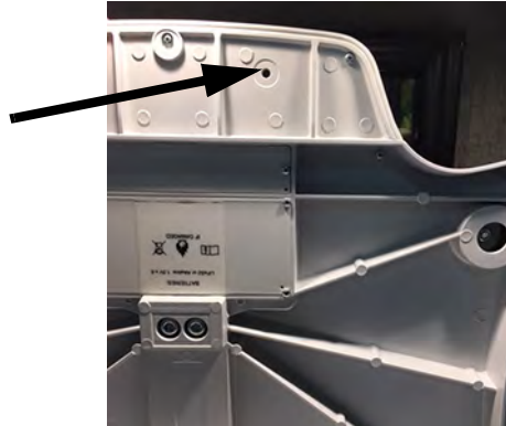
Figure 3-1. Setup Switch Location
