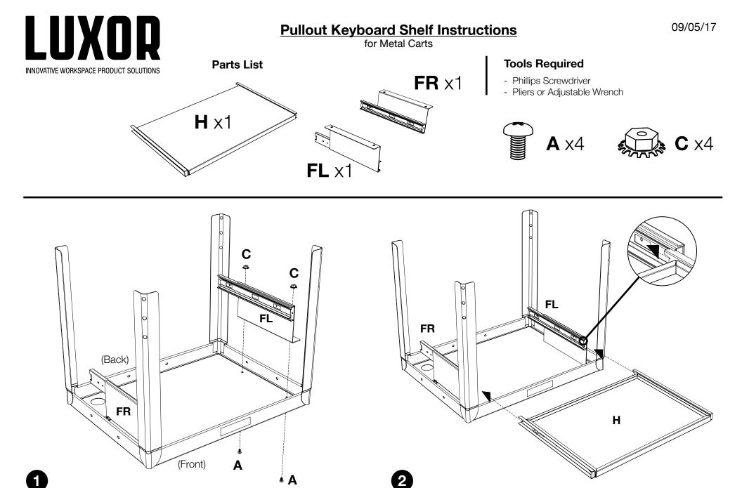
Take the top shelf of your metal cart and lay it flat. Collect parts: **FL**, **FR**, **A** & **C**. Push Screw **A** through the hole at the top of the shelf. Lay bracket **FL** & **FR** on top of screw **A**. Take nut **C** and fasten with a screwdriver and pliers, do not tighten fully until shelf is attached.
