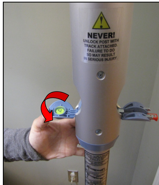
Step 7: Swing open post level. Please ensure the level is fully open.
