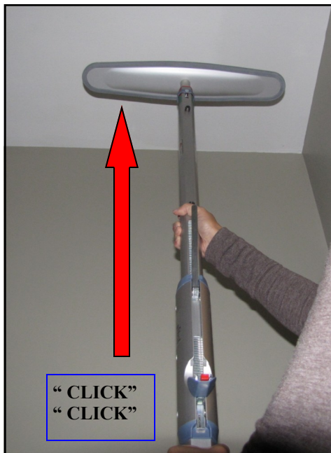
Step 6: Push the top section of post up towards the ceiling with Top foot. Upon contact with the ceiling, continue pushing up until you hear one or two more “clicks”.
