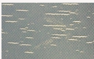
Magnified view of mattress covers damaged by chemicals and abrasion where "strikethrough" damage is starting to occur*
