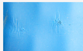
Magnified view of mattress covers damaged by chemicals and abrasion where "strikethrough" damage is starting to occur*
