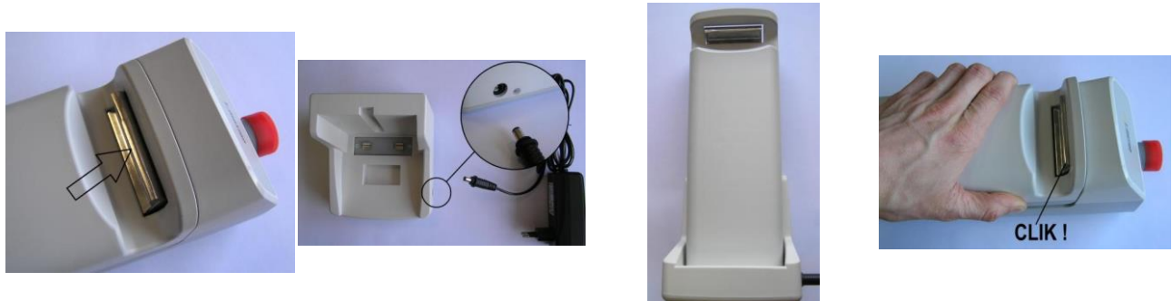
Figure 15 - Charging and handling the battery
