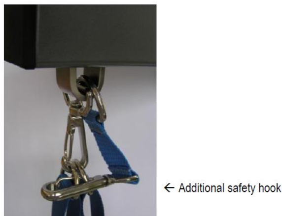
Figure 7 - Mounting the harness to the weight bearing arm
