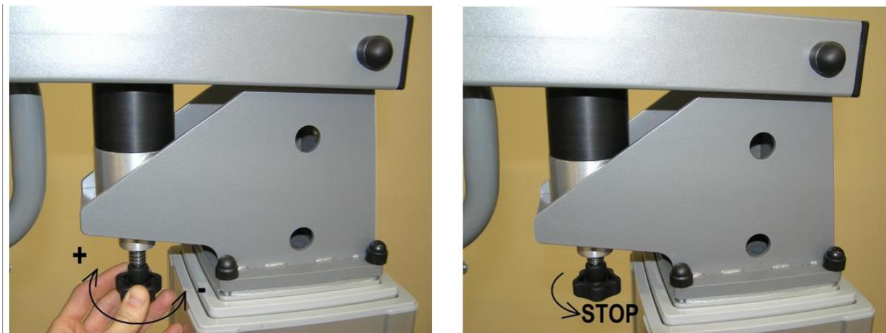
Figure 3 - Adjusting dynamic partial weight bearing system
