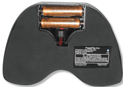
Figure 2: Battery cover is located at the bottom of the PageFlip Cicada. A convenient storage compartment for the Bluetooth dongle lies alongside the batteries.
