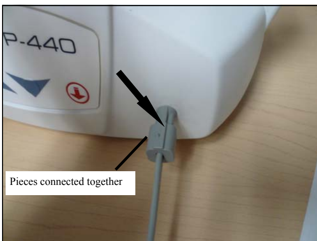
Figure 15C - Gray rubber airline being inserted into rubber grommet of lift. The ridges on both pieces are lined up. The metal ribbed pins are on the airline.
