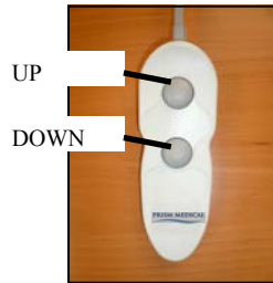
Figure 4A - Methods to Turn the P-440 "ON"
