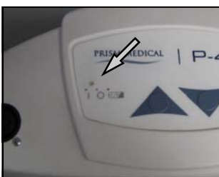
Figure 4B - The indicator light of the lift is normally off when not in use.
