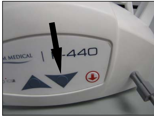
Figure 14A –Lift showing DOWN button located on front right side of lift.
