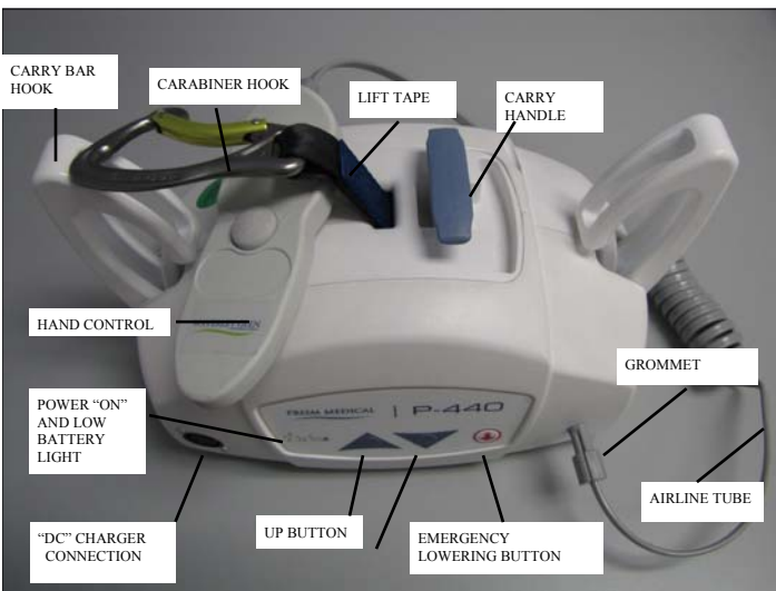
Figure 2A - Front View of P-440 lift
