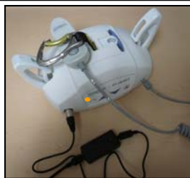
Figure 12C - Close-up of "DC" charger plug and lift "DC" charger connection. Note the 3 metal prongs on the end of the charger cord and 3 holes on the black "DC" connection.
