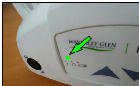
Figure 4C - When the lift has been turned "ON", the indicator light will turn green.
