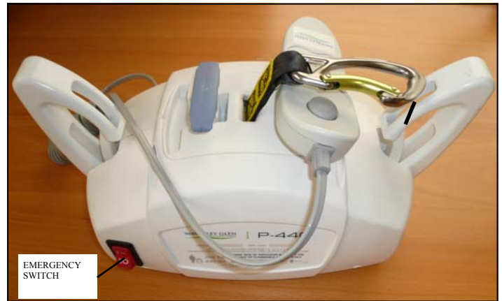
Figure 2B - Back view of P-440 lift
