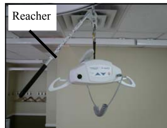
Figure 9A - Photo showing P-440 lift carabiner connected to a reacher first and then to the eyelet of the trolley.
