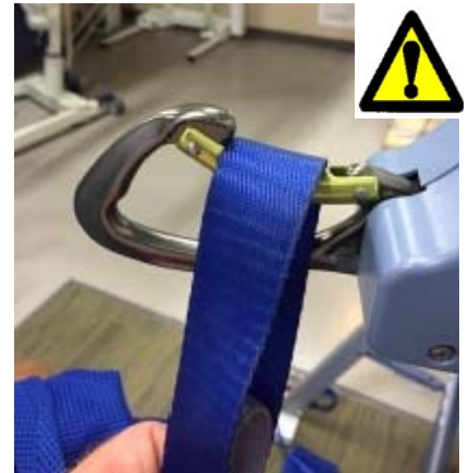
Sling loop flipped over and incorrectly resting on the latch.
