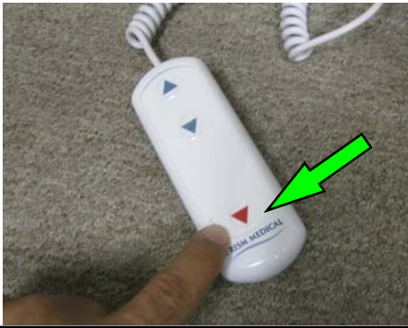
Figure 14A –RED emergency lowering button located on bottom of the hand control.
