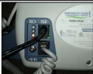
Figure 12E - Charger is connected to the lift. The 2 green indicator lights on the unit will start blinking showing actual status of recharge. Top two Led’s will turn solid “Green” once charging is completed.
