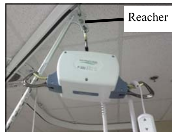
Figure 9A - Photo showing P-300 lift carabiner connected to a reacher first and then to the eyelet of the trolley.
