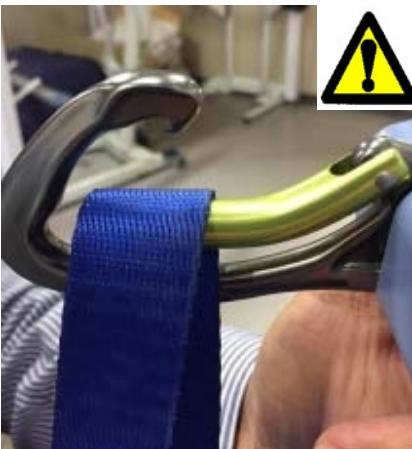
Load applied. The sling loop begins to slide off the latch.
