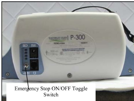
Figure 14C –RED Emergency stop switch located on the front left side of the lift.
