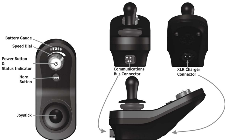
Figure 37: The Remote REM060: user interface and connectors
