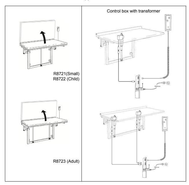
**Installation location** This product is designed for indoor use in a wet environment, such as a bathroom or washroom, therefore, ensure that the power supply is adequately shielded. Additionally, choose an installation location with sufficient space for access to and function of the product.
