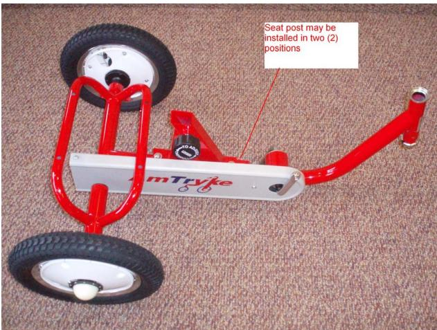
NOTE: THE SEAT POST ASSEMBLY MAY BE MOUNTED IN TWO (2) POSITIONS ON THE FRAME. THIS ALLOWS DIFFERENT POSITIONING BASED ON THE RIDERS SIZE. THE SEAT COMES MOUNTED IN THE BACK SET OF HOLES FROM THE FACTORY.
