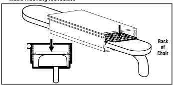
The Snap Tabs on either side of the Sliding Spacer MUST BE INSTALLED INTO THE SAME SLOT ON EACH SIDE OF THE BRACKET.
