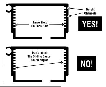
To remove the Sliding Spacer, gently squeeze both Snap Tabs in, and push the Sliding Spacer back through the bracket.
