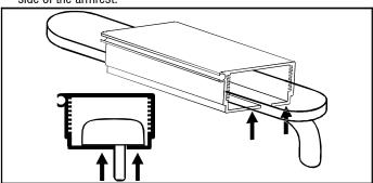
3. To insert the Sliding Spacer into the appropriate Height Channel, put the Snap Tabs in a channel, then push the Sliding Spacer completely into the bracket so that the tabs go completely through the bracket and snap into place. This allows the Sliding Spacer to be locked in place. NOTE: To choose the correct Height Channel, choose the channel that will allow the bracket to snugly fit on the armrest pad. The bracket must fit snugly on the armrest to provide a stable mounting foundation.
