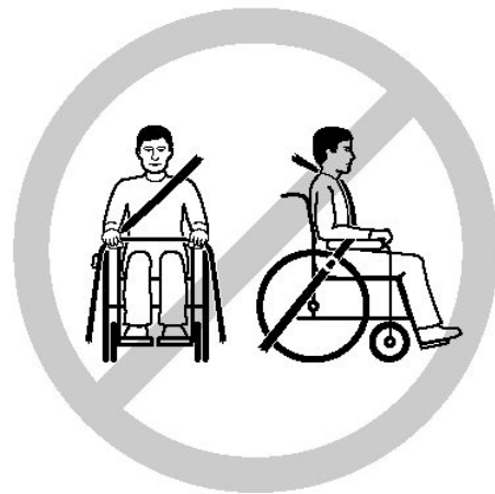
Incorrect seat belt position
