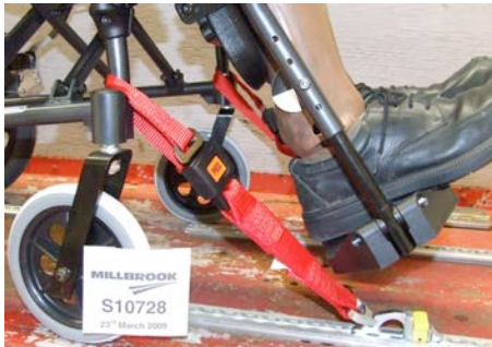
Fitting the front restraint
