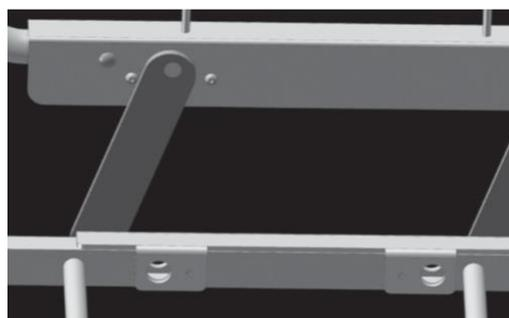
5. Re-insert the metal pins from the outside edge of the bed through the mounting holes and secure with snap rings on the inside edge of the bed. Make sure the snap rings are positioned in the groove of the metal pins.
