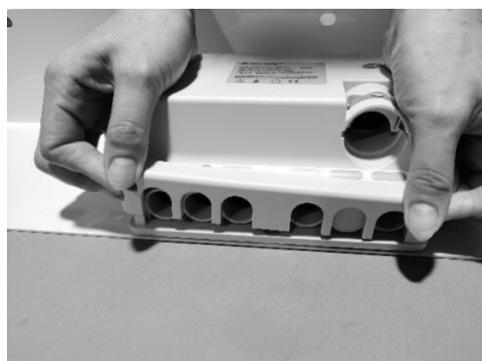
3. Open the control box locking lid by pressing in the sides and lift it up, to expose the connection ports.
