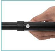
6. Screw the (E) Nuts onto each of the four bolts so that the bolts are secured, again make sure the hexagon shaped heads of the bolts fit snugly into the hexagon shaped holes.
