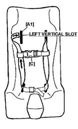
5> Then bring the web end [A1] through the other side of the chest strap [C] and through the left vertical slot.
