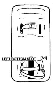
4> Bring the strap around the back of the seat and through the left bottom slot.
