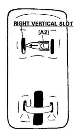
2> To attach the long strap take web end [A1] and thread it from the back of the seat through the right vertical slot. Make sure buckle [A2] is facing outward.
