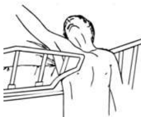
Entrapment between split bed rails
