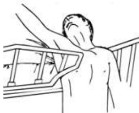
Entrapment between split bed rails
