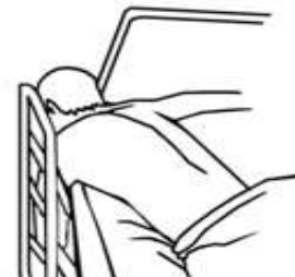
Entrapment between the end of the rail and the side edge of the headboard or foot board
