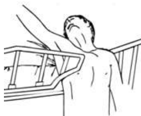
Entrapment between split bed rails
