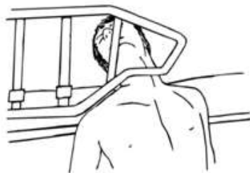
Entrapment under the bed rail at the ends of the bed rail
